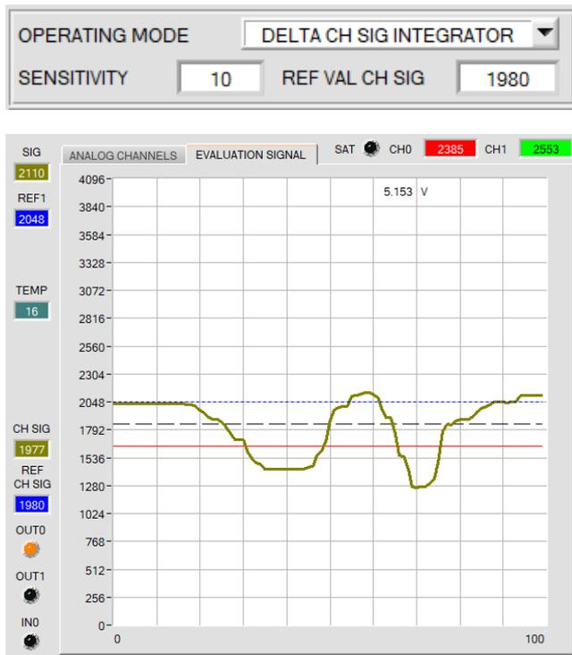
With **DELTA CH SIG INTEGRATOR** the deviation of **CH SIG** from a reference value for **CH SIG (REF VAL CH SIG)** is determined, standardized to 4096 and added with 2048.
